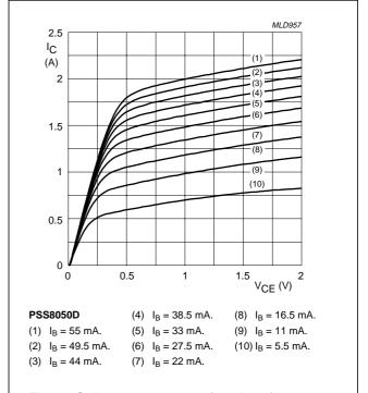
Fig.13 Collector current as a function of collector-emitter voltage; typical values.
