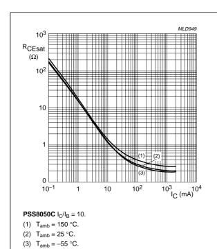
Fig.6 Equivalent on-resistance as a function of collector current; typical values.
